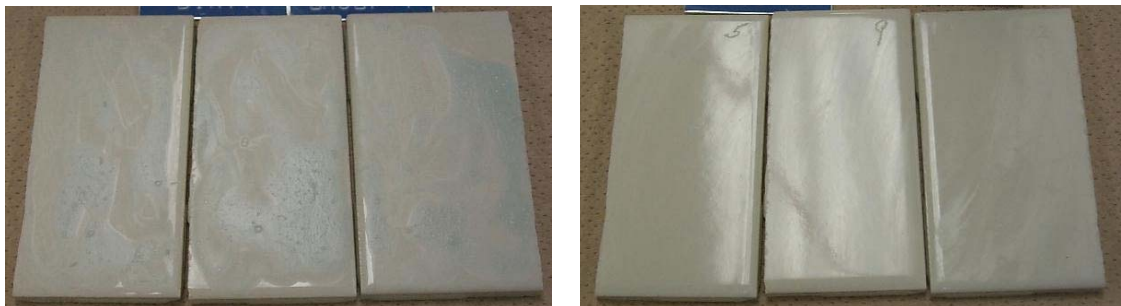
Figure 9. PHOTOGRAPHS OF CERAMIC BEFORE (LEFT) AND AFTER (RIGHT) GENERAL PURPOSE CLEANING
