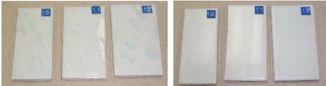
Figure 2. PHOTOGRAPHS OF CERAMIC BEFORE (LEFT) AND AFTER (RIGHT) GENERAL PURPOSE CLEANING
