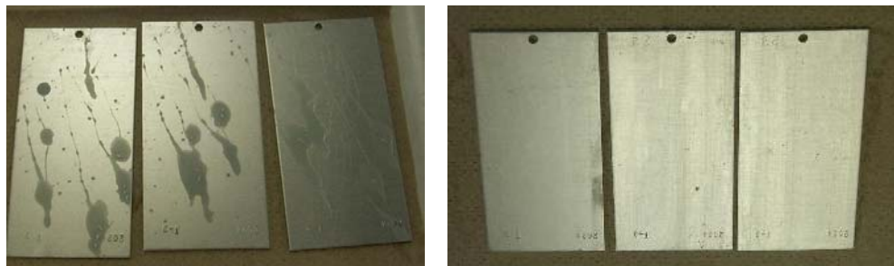
Figure 3. PHOTOGRAPHS OF CHROME BEFORE (LEFT) AND AFTER (RIGHT) GENERAL PURPOSE CLEANING
