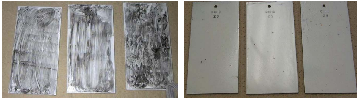
Figure 8. PHOTOGRAPHS OF STEEL BEFORE (LEFT) AND AFTER (RIGHT) GENERAL PURPOSE CLEANING
