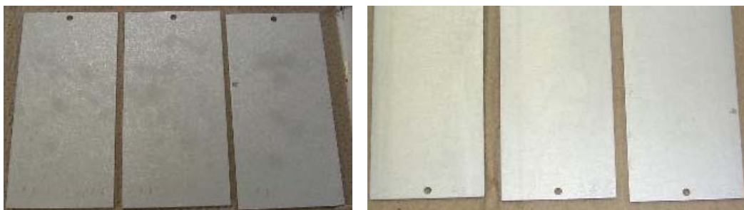
Figure 5. PHOTOGRAPHS OF CHROME BEFORE (LEFT) AND AFTER (RIGHT) GENERAL PURPOSE CLEANING
