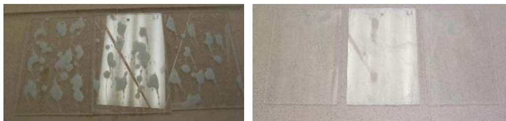
Figure 1. PHOTOGRAPHS OF FIBERGLASS BEFORE (LEFT) AND AFTER (RIGHT) GENERAL PURPOSE CLEANING
